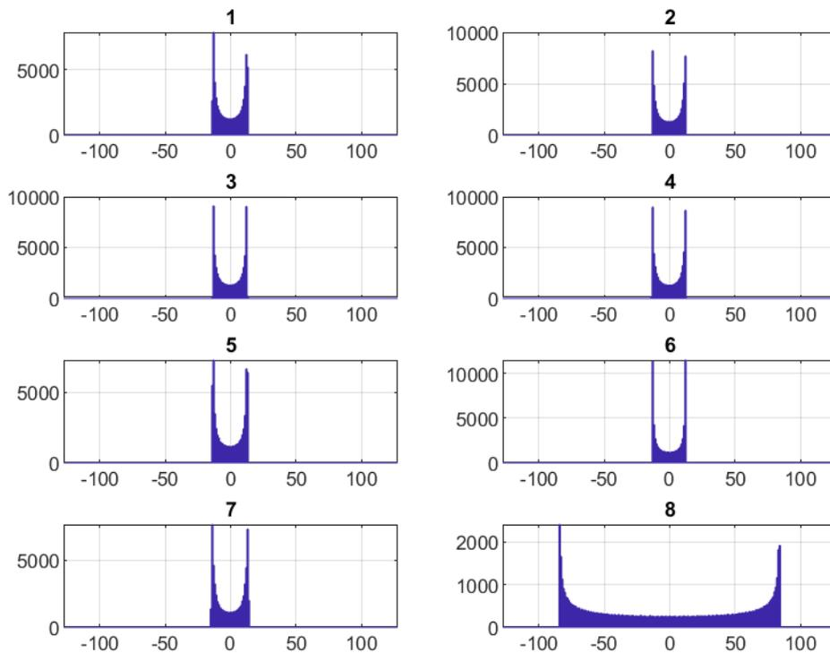
Figure 2: Typical set of histograms of the 65,536 samples from the 8 channels of two ADC devices. Channels 1-4 (B1-B4) are coax-connected and 5-8 (D1-D4) are differentially connected via ARJ45. In this case, the 34 MHz test signal was driving channel 8 at an amplitude of about 80 ADC counts, and the other channels were driven by the 97 MHz dither signal at an amplitude of about 8 counts.
