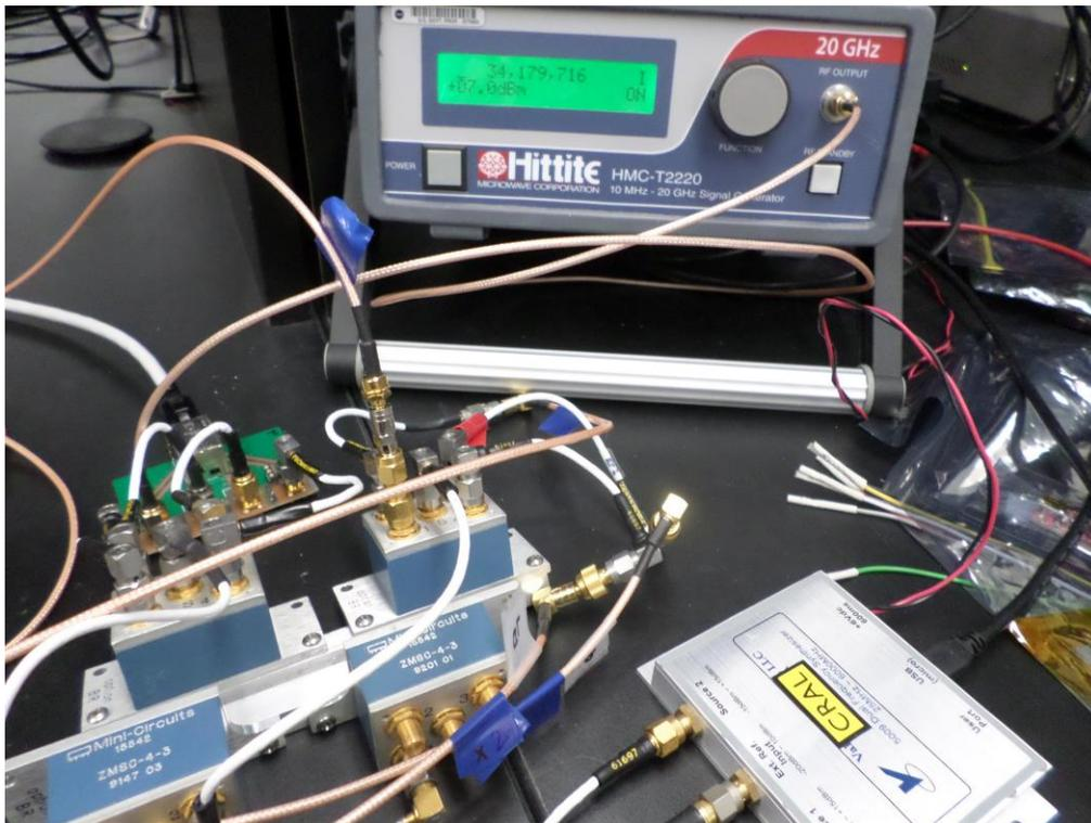
Figure 1: Photograph of part of the test setup. in the right foreground is the Valon 5009 synthesizer, and on the left is a set of four 1:4 power dividers (1 unused) for dividing the dither signal among 7 ADC inputs. Behind the power dividers is the SMA-to-ARJ45 breakout board.
